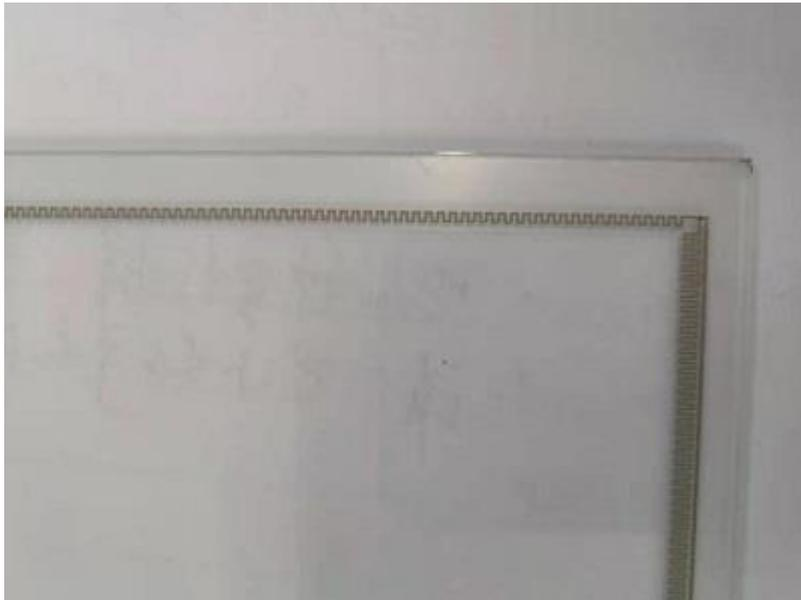
The above pattern edge is typical for the current market, however this can only achieve resistance within the range of 50 ohms. Smaller size touchscreens, the resistance will even be lower. Our design can provide for 50-200 ohm resistance which eliminates issues that occur with touch controllers.
