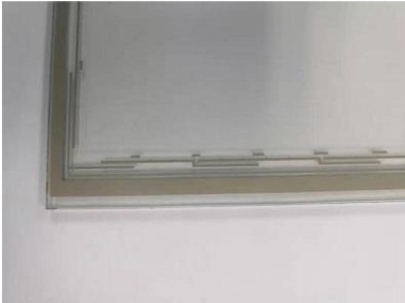
Above is another pattern available in the market. Due to existence of contact point in between the edge and sensitive area, this design creates a wave near the edge, affecting the contact around the perimeter of touch screen, reducing the available useful touch area.
